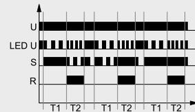
The input of the time relay is supplied with voltage U continuously. Closing of the control contact S starts the interval T1, and after the interval has lapsed, the output relay R switches on for the interval T2. Following the interval T2, the output relay switches off, and the circuit awaits for the control contact S to be closed again. In the course of the intervals T1 and T2 the position of the control contact S is of no importance.
